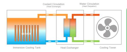
Single-phase direct immersion liquid cooling design, the server is completely immersed in fluoride liquid or mineral oil, and the chip heat is brought out to the heat exchanger through the excellent flow path design, and then the heat is brought to the cooling tower and other heat dissipation facilities through water circulation, which can achieve year-round free cooling, greatly saving cooling costs and improving server power density.
