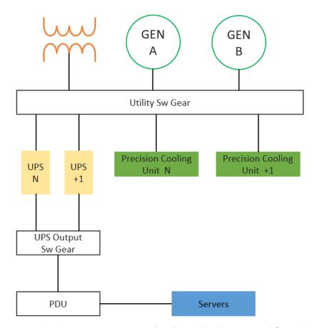
**Availability:** Lower, redundant components can be planned to be removed for maintenance without causing IT equipment to shut down, but unplanned equipment or distribution path failures can cause IT equipment to shut down.
