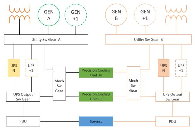
**Availability**: The highest, any single infrastructure equipment and path failure will not cause service disruption, and can be maintained online.
