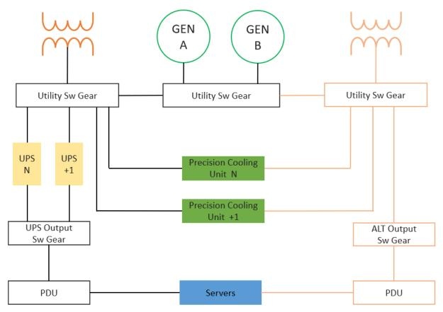
**Availability:** High, all single components and distribution paths can be systematically removed from the system without affecting any critical environment, but unplanned failures can cause IT equipment to shut down.
